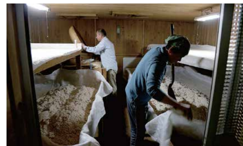
Making koji. Koji is made by sprinkling spores on steamed rice in the stone koji room and takes 42 to 44 hours to complete. The koji is then moved to clay pots buried in the ground to make the mash.
