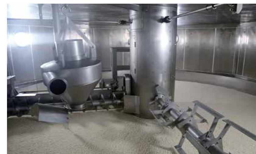
A giant rotating koji production chamber, capable of holding three tons of koji. This facility controls the temperature and humidity inside, producing massive amounts of koji. This is just one example of how mechanization has evolved to maintain quality at pace with the increase in output.
